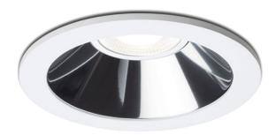
The Burst is a Ø188mm large area downlight aimed at low glare environments (UGR <19). The downlight only requires 80mm of ceiling void making it ideal for installations where space is tight. The Burst can achieve a lumen package of up to 2,200lm with a longevity of at least 60,000 hours.
