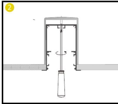
1. Offer up the profile with clamping arms folded in through the cutout pre-made in the ceiling. We Advise to have power feed be terminated into the gearbox at this point (see the wiring diagram on the next page).
