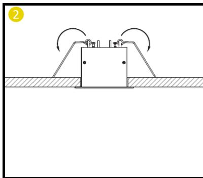
1. Terminate the power feed to the luminaire gearbox (see the wiring diagram on the next page) and offer the luminaire up to the ceiling with the spring arms pulled back.
