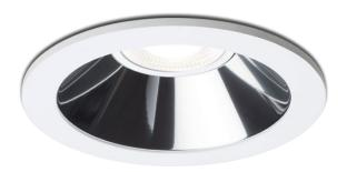
The Burst is a **Ø**188mm large area downlight aimed at low glare environments (UGR <19). The downlight only requires 80mm of ceiling void making it ideal for installations where space is tight. The Burst can achieve a lumen package of up to 1,724lm with a longevity of at least 60,000 hours.
