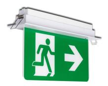
The Shield RCD (Recessed) is a 3 Watt LED exit sign for use in MF and fibre tile ceilings. The RCD version of the Shield finishes flush with the underside of the ceiling plane for minimal intrusion of the space. The unit is available in Maintained and Non-Maintained modes.
